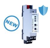
Compact KNX / modbus gateway with 250 freely configurable channels (KNX data points). The device allows easy integration of modbus devices supporting the RTU protocol via RS-485 into KNX installations. It can be used as modbus master or slave. The assignment between KNX objects and modbus registers is done via parameters in the ETS® - no further tool is required. With 2x pluggable screw connectors. One connector can be used with Modbus for the terminating resistor.
