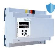
The device combines the central functions of a KNX bus line: Bus power supply with bus choke, KNX IP router and KNX IP interface with low space requirement. Comprehensive diagnostic functions. The KNX IP router in the LineMaster enables the forwarding of telegrams between different lines via a LAN (IP) as a fast backbone. The device also serves as a programming interface between a PC and the KNX bus (e.g. for the ETS®).
