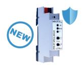
KNX IP interface to the KNX bus, both at telegram level (KNXnet/IP tunnelling) and at data point level (KNX application layer). This allows clients to access group objects directly via TCP/IP using a binary protocol. The device supports KNX Security and BAOS Security.
