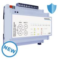
Compact KNX switching actuator with central power supply and 12 outputs. Functions for universal output, staircase lighting, heating actuator, etc. Optimised for LED lights.
